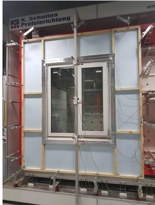
Figure 5. General view of the PVC window installed in the test stand for the combined wind and temperature load action.
