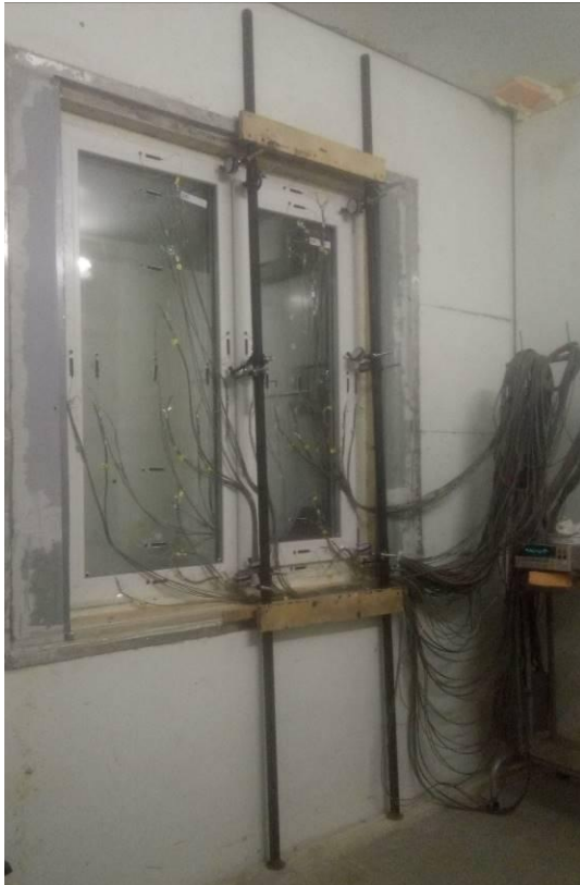
Figure 4. General view of the PVC window installed in the climatic chamber for testing the temperature load.
