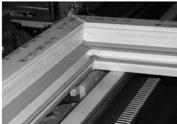
Figure 3. Corners received in welding process
