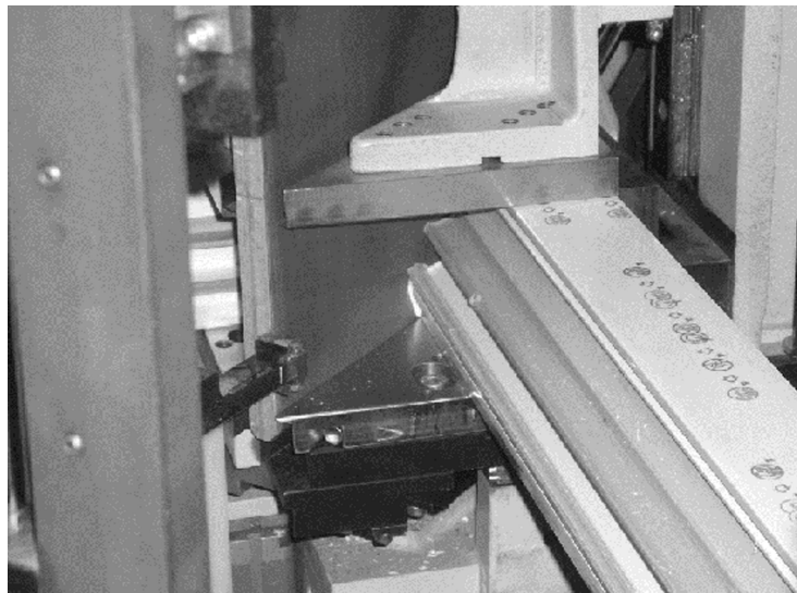
Figure 2. Fusing-in the profiles' edges before welding process
