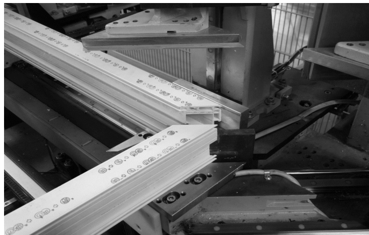
Figure 1. The view of welding station presenting the arrangements of the components before starting the process
